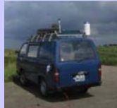
Fig. 1: Mobile platform on which the X-Band radar is mounted
