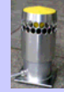
Fig. 3: Joss-Waldvogel - Disdrometer which is mounted on the roof of the radar van.
