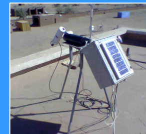
CLIMAT : a 4 channels IR Radiometer: 8-13 \mu\text{m} , 8.2-9.2 \mu\text{m} , 10.3-11.3 \mu\text{m} , 11.5-12.5 \mu\text{m}
