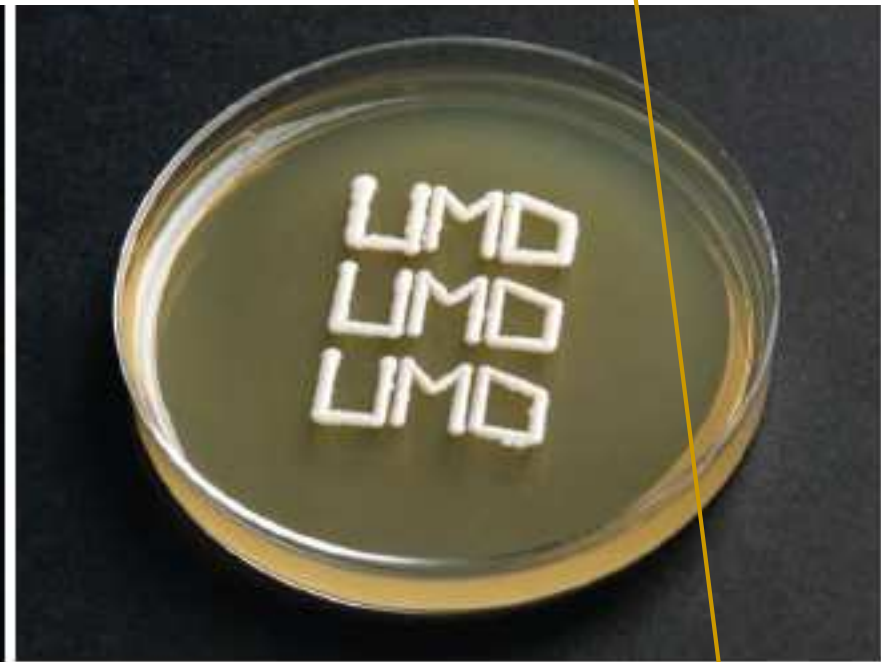
Cells on demand. (Left) Three-dimensional tube structure made from bioprinted cells. This composite image shows an inner layer of human umbilical endothelial cells (green) and an outer layer of human aortic smooth muscle cells (red). (Right) Printed and cultured yeast patterns after 3 days of culture. The patterns were printed at 75, 150, and 300 drops per second, from top to bottom.
