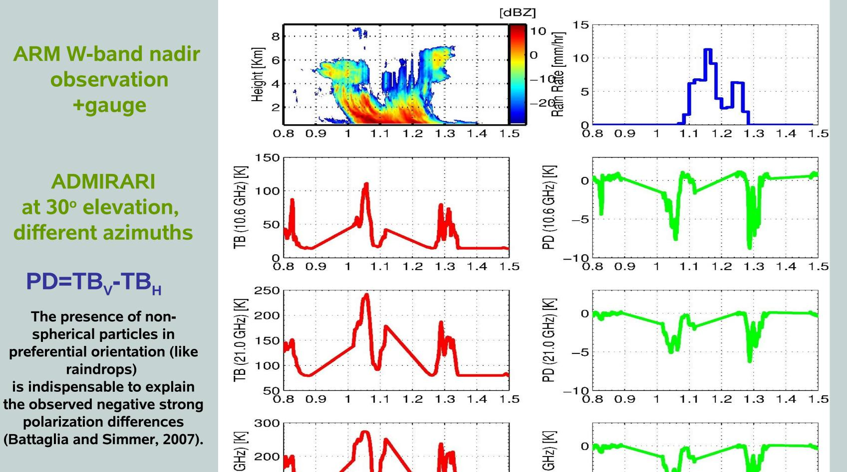
The higher frequency channels (21-36.5 GHz) saturates for high/medium rain rates. PDs are lower than at 10 GHz (as expected from theory, Czekala et al, 2001).
