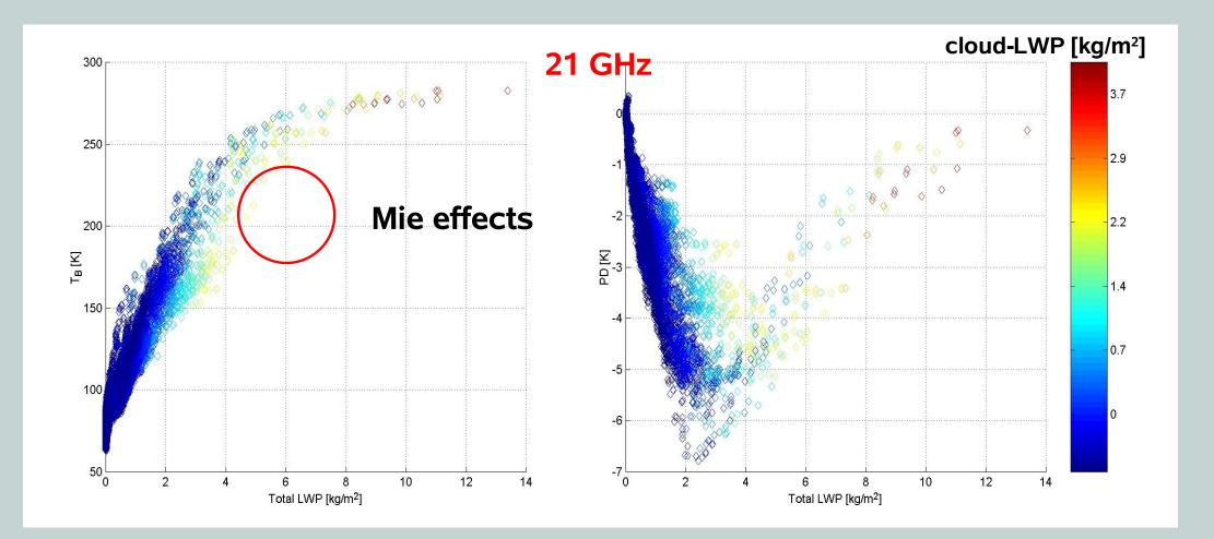
A database of TBs and PDs and corresponding hydrometeor profiles has been created. This will represent the core of the physical retrieval algorithm.
