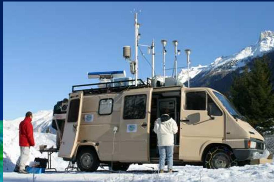
Scanning Lidar + aerosol sampler
