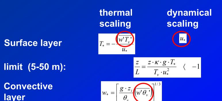
Remark 1: Coherent structures are already generated in the surface layer. There is a connection to such structures in the boundary layer. Remark 2: There is no remote sensing technique available to determine these parameters.
