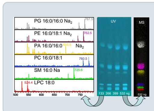
**Fig. 3:** Detectability of HPTLC-MALDI: A dilution series of lipid standard containing 133-532 ng of each lipid was analyzed. Even at the 133 ng level intense MALDI spectra were obtained that can be well interpreted. Parent ion masses refer to MH<sup>+</sup> or sodiated peaks.
