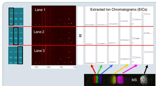
**Fig. 2:** Repeatability of HPTLC-MALDI. 3 repetitive analyses with 330 ng lipid standard on 2 TLC plates were developed by primuline (left) and MALDI (center). Repeatability of the intensities of extracted parent ion chromatograms (right) is **better than 10 %**.
