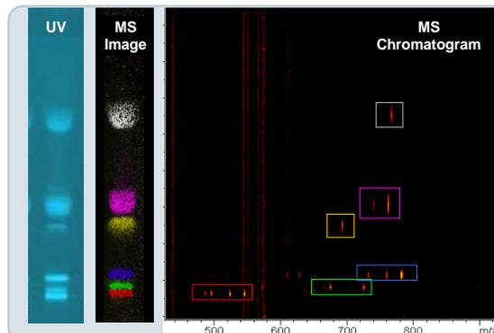
**Fig. 1:** HPTLC analysis of 532 ng of a lipid standard mixture: (UV) primuline, fluorescence at 366 nm; (MS Image) MALDI-TOF image analysis, false color representation of ion distribution; and (MS Chromatogram) heat map mass chromatogram with lipid signals (Rf vs. m/z) boxed corresponding to the MS image. The chromatographic representation provides a 2D high resolution access to TLC-MALDI data. DHB was used as MALDI matrix.
