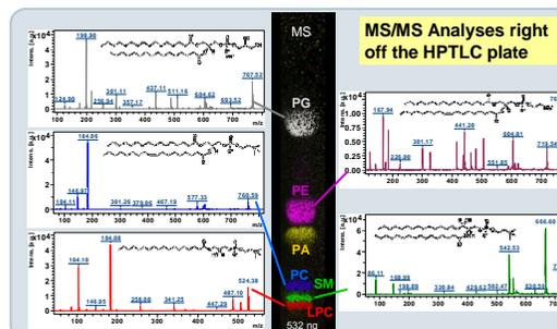
**Fig. 4:** Structural elucidation Software supported MALDI-TOF/TOF MS/MS spectra acquisition right from the HPTLC plate after MS acquisition. Fragment ions correlate with the respective lipid structure and permit its unequivocal identification and head group assignment.
